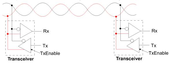
Each node uses a *transceiver* that consists of a differential receiver and differential driver whose legs are connected together on the "plus" and "minus" sides. When the node is "listening" the driver TxEnable is deasserted putting the driver into a high impedance tri-state mode. When the node needs to transmit, the driver TxEnable is asserted, applying the Tx state to the differential bus. This means that only one driver can be asserted at any time.
