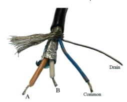
common wire is landed on each isolated ground terminal. The drain daisy-chains through cabinets but is only grounded at one point.
