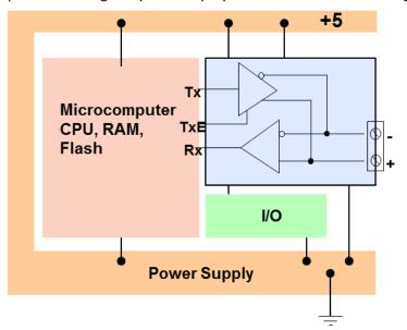
The Microcomputer, memory, Input/Output (I/O) and EIA-485 components share access to a power supply circuit that provides appropriate voltage(s) all of the individual components. Of particular interest is that the ground reference for the entire device is the same as the power supply ground.
