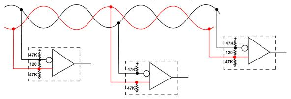
Since the standard allows both types of biasing philosophy there is always the possibility that a given MS/TP segment may include a mixture of types. For network segments containing 32 or fewer nodes that is not a problem. However, when you want to have the same MS/TP segment include more than 32 nodes, the biasing philosophy becomes very important.
