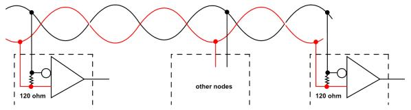
The standard also requires that both extreme ends of the network bus shall have  $120\Omega$  termination resistors across the receiver. Termination is important over longer distances and higher speeds to eliminate reflections.
