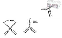
outgoing wire ends rattail fashion and capturing the twist in the corresponding screw terminal for the network. Be sure not to expose too much bare twisted wire so that adjacent wires don't short, or use crimp sleeves.
