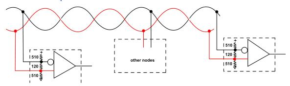
The extreme end nodes of the network bus are enhanced to include *pullup and pulldown biasing* resistors. The values chosen for these resistors must be small enough to provide more than 200mV of voltage drop across each receiver, and large enough that they do not exceed the driver's ability to overcome the bias which would prevent transmitting data. MS/TP specifies the use of  $510\Omega$  resistors for end point (network) biasing.
